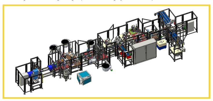
**Zone 1 - Initial Loading and Pre-Assembly:** The operator manually loads components inside a rotofriction welder. After the gasket is added, the part is placed on a pallet that begins its advancement down the line. The area is protected by an intangible barrier and interlocked movable guards, which allow safe intervention if necessary;
