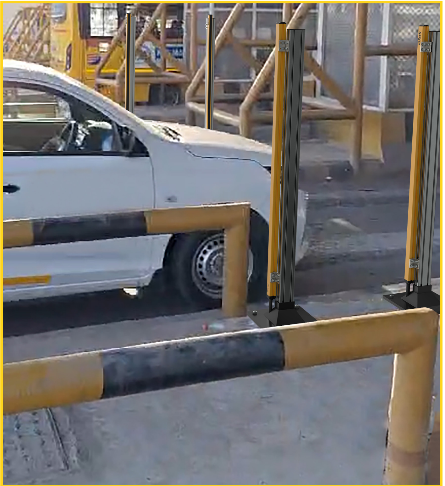
In the picture, the pair of EOS safety light curtains for vehicle transit detection and speed control.
